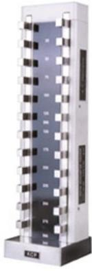
This Depth Micro checker is designed for efficient calibration and zero setting of Depth Micrometers
