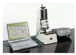
Gauge Block Comparators are specifically designed for the measurement of Gauge Blocks by comparison, with no compromises made.
