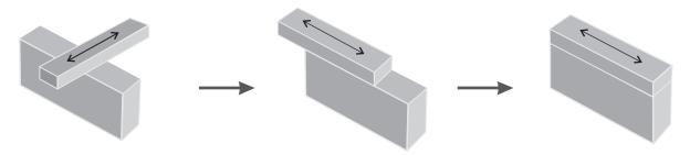
Bring the two measuring faces of gauge blocks into contact with each other at right angles.
