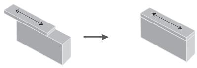
Place one end of thin gauge block on the closer end of thick gauge block.
