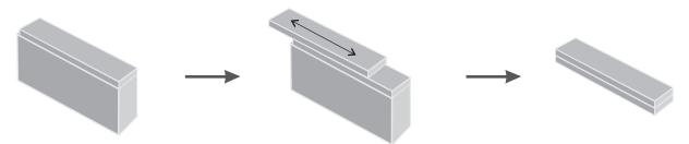
To prevent thin gauge block from bending, take a thick gauge block, first wring thin gauge block on the thick one. Then wring other thin gauge block over the previous thin gauge block.
